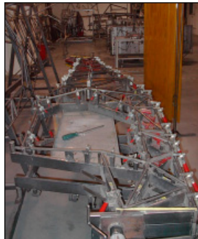
Taking a close look at the one of the KitFox fuselage jigs.
