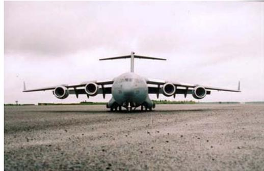
The model also has smoke systems both of the inboard turbines, and uses 2.4 GHz data link to provide real-time data to a laptop computer on the ground while in flight, this data includes airspeed, turbine RPM, EGT, fuel consumption, etc. It is covered in fiberglass and epoxy resin. Built mainly from balsa and ply, with many glass and carbon fiber moldings to reduce weight.
