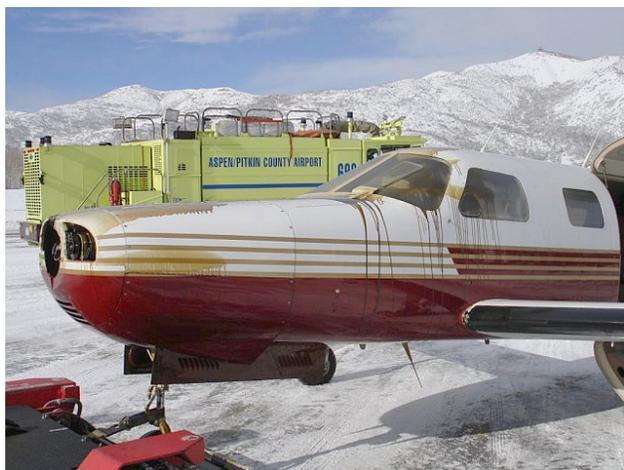
**This Piper Malibu recently developed severe vibration, 'low oil pressure and a possible oil leak' several miles out from Aspen. The pilot managed to land despite an oil-coated windshield obscuring forward visibility. He later found the entire prop had 'departed' in flight**
