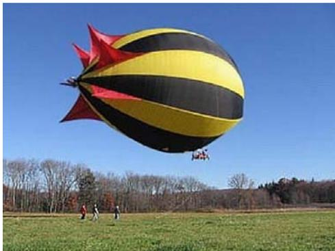
Called the Alberto, after Brazilian aviation pioneer Alberto Santos-Dumont, it is 102 feet long, 70-feet in diameter, uses hot air for lift and has a tail propeller for precise directional control.
