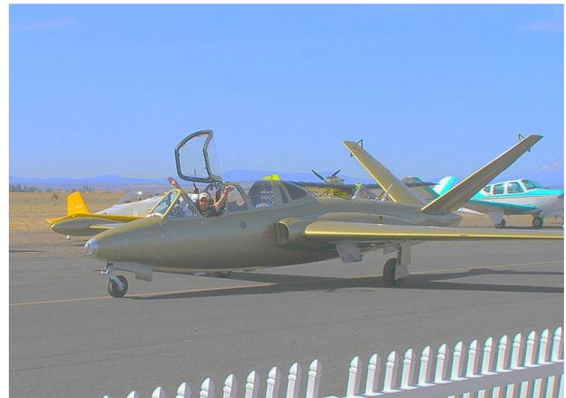
In 1948, French aircraft manufacturer Fouga designed a jet-powered primary trainer called CM.130 for the French Air Force (Armée de l'Air, AdA) to replace piston-engined Morane-Saulnier MS.475 aircraft. When AdA found the aircraft lacking in power from the two Turbomeca Palas turbojets, Fouga enlarged the basic design and used the more powerful Turbomeca Marboré engine.
